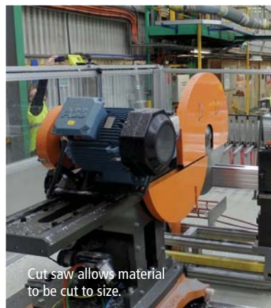
Designed to machine up to 17m lengths of aluminium profile.
