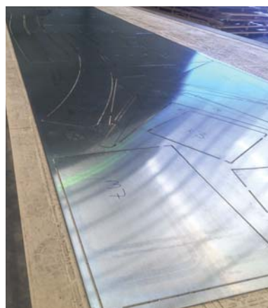
Material optimisation through effective nesting of cut parts, maximising yield and minimising waste.
