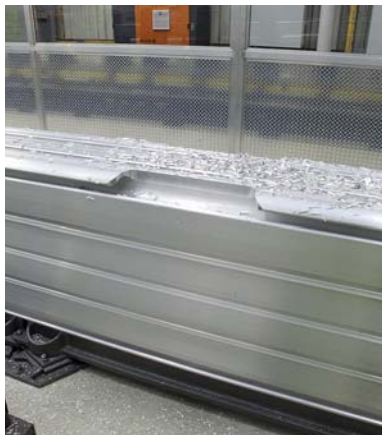
Designed to machine up to 17m lengths of aluminium profile.
