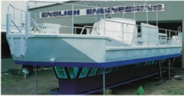
The first of a new generation of reef viewing boats where passengers sit below water level
