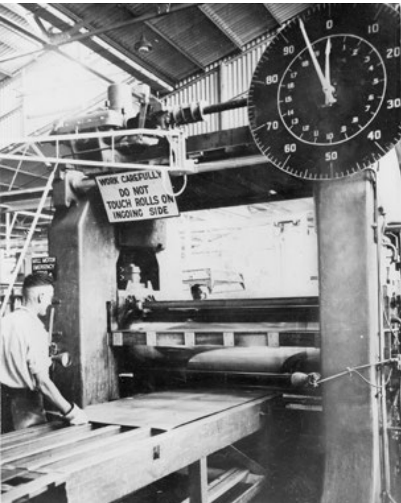
Aluminium sheet being hot rolled at the Australian Aluminium Company in Granville, New South Wales, around 1942. H4882-1, 14, 25, Collection: Powerhouse Museum.
