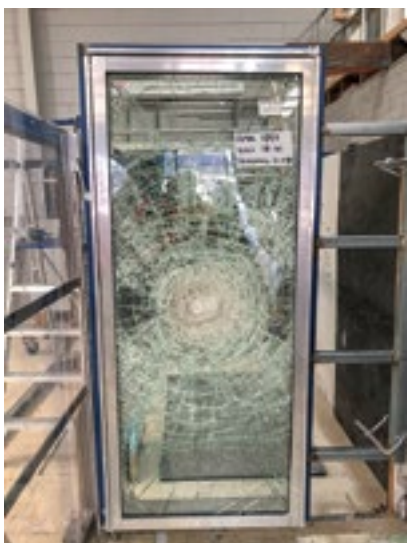
The aftermath of Cyclone impact testing
