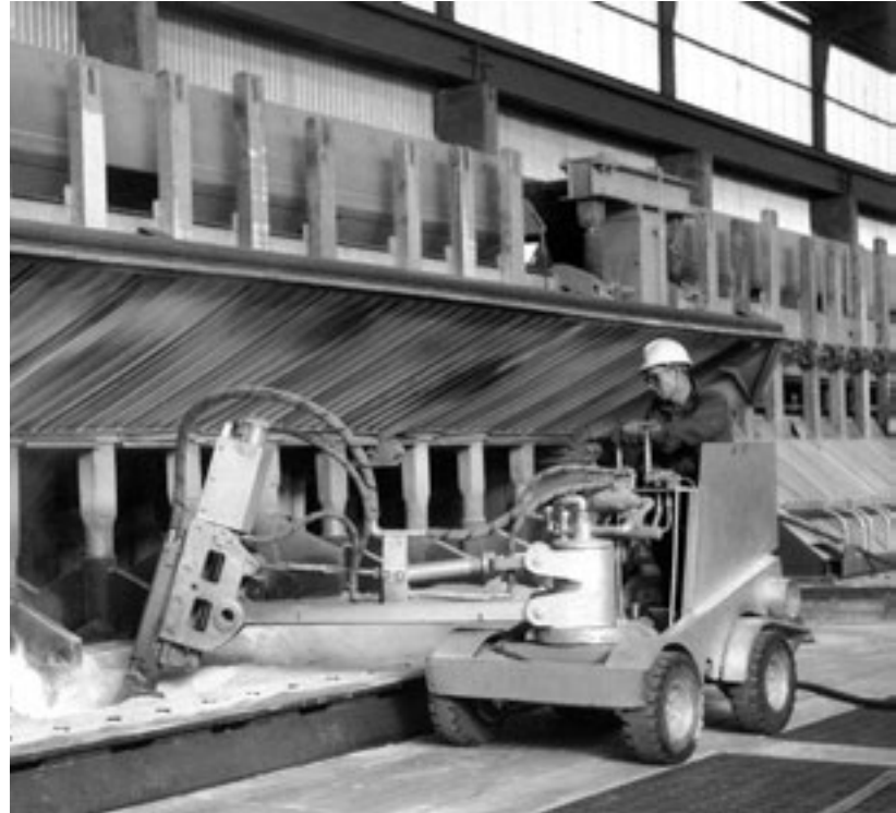
Cryolite being cleared from potline anodes
