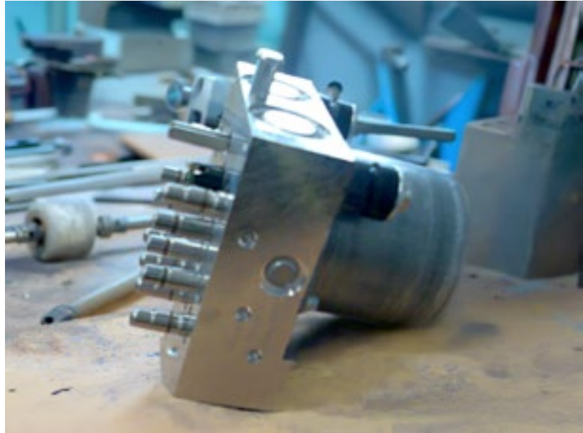
Aluminium ABS brake housing made for Bosch
