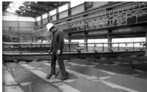
Checking anode baking
