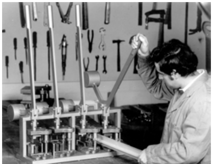
Early press tool used to perform punching operations on window and door sections, 1980s
