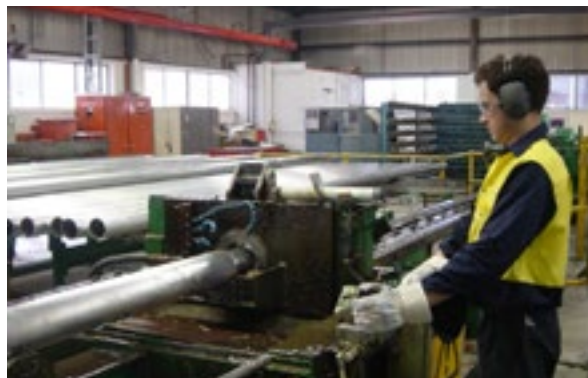
Cold drawn process - achieving the overall tolerances for driveshafts and torque tubes.
