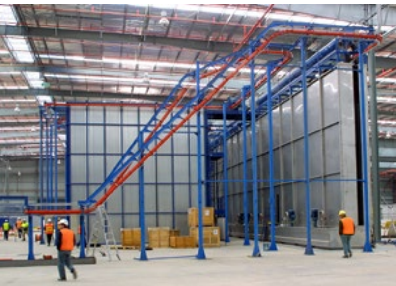
Stretch line refurbishment (top right), new control panel for press (middle), vertical powder coat line (bottom), 2004
