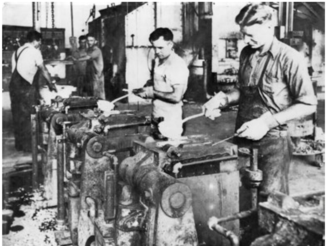
Aluminium being sand cast at the Australian Aluminium Company in Granville, New South Wales, 1940s. H4882-1, 14, 25, Collection: Powerhouse Museum.
