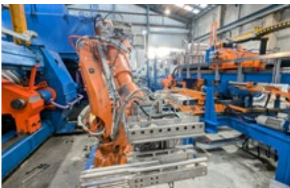
World first robotic billet loading at the newly modernised press
